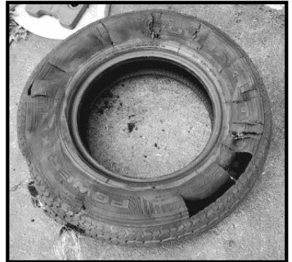
Figures 1 & 2: Examples of tire failure due to overloading:
