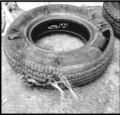
Figures 1 & 2: Examples of tire failure due to overloading:
